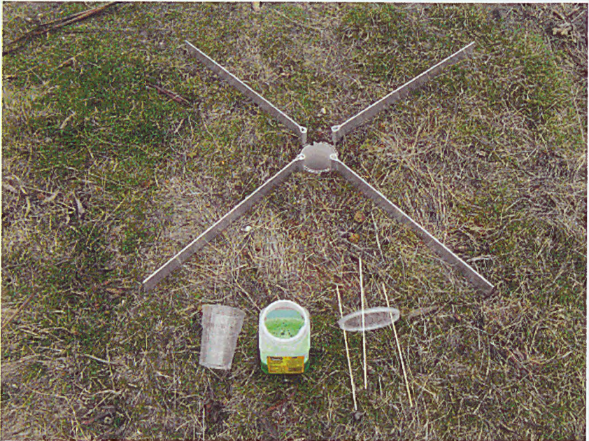
Fig. 2. The components of the guide-arm trap include: the directing arm brackets attached to the metal collar and trap tube, collection cup, preservative (ethylene glycol) and rain cover.
